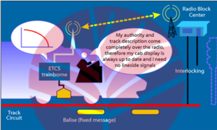
Fig. 3.20: ERTMS level 2. Source: ERTMS website
